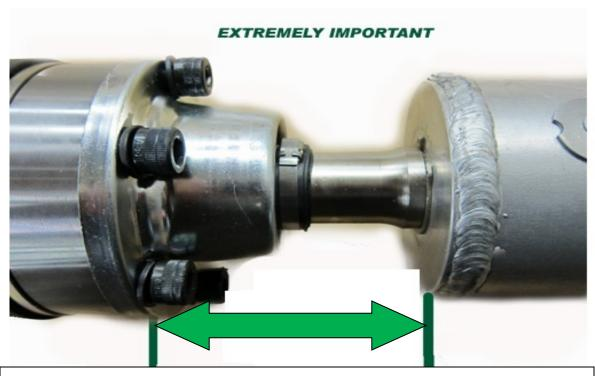
Driveshaft CV Clearance MUST BE CHECKED after installation. BMW E36 / E46 M3 must be between 3.25'' - 3.75'' If dimension is not within the allowed range, do not run the driveshaft
