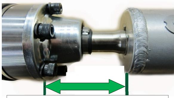
Driveshaft CV Clearance <u>MUST BE CHECKED</u> after installation. 1993-1998 Supra (Auto / Manual) must be between <u>3.25" – 3.75"</u> If dimension is not within the allowed range, do not run the driveshaft
