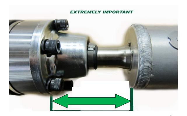
Driveshaft CV Clearance <u>MUST BE CHECKED</u> after installation.
