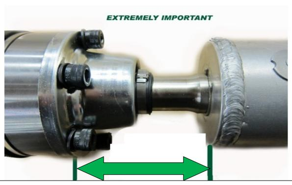
Driveshaft CV Clearance <u>Must BE CHECKED</u> after installation. If dimension is not within the allowed range, do not run the driveshaft
