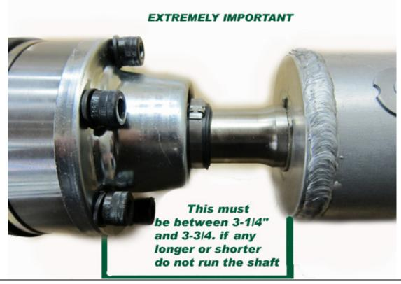
Please Note: The included 6-bolt CV adapter plate MUST be installed onto the factory differential flange before the driveshaft can be installed. This is not an optional part, nor is it a spacer as the bolt pattern on the DSS CV and the factory differential flange are not the same.
