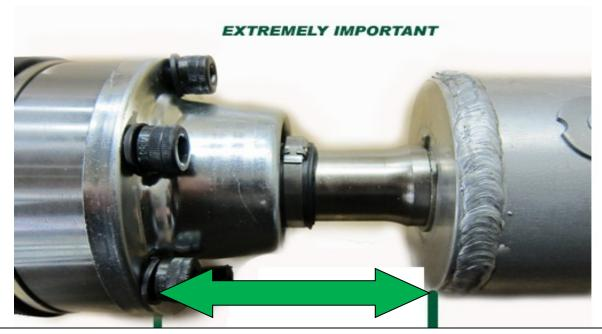
Driveshaft CV Clearance <u>MUST BE CHECKED</u> after installation.
