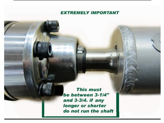
Please Note: Vehicles with a live rear axle (2005-2014 Mustang) must be checked with the rear suspension set at ride height.
