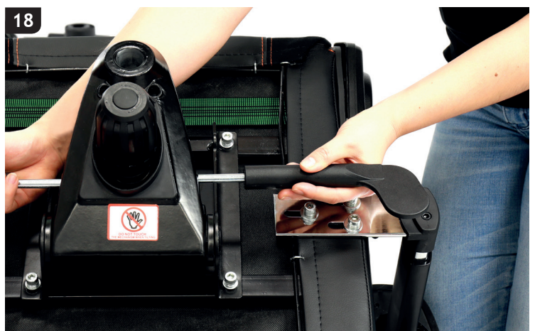
18 Place the handles on the tilt mechanism's axles. The rounded edge of the handles should point towards the front of the seat bottom.
