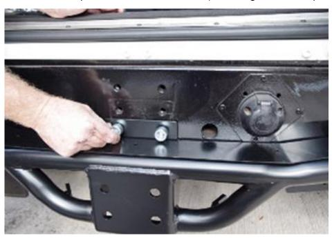
8, Fix bracing bars from NAS to chassis with 4 M12 x 50mm with nuts
