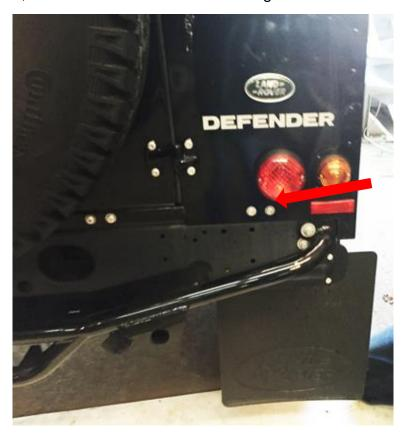
5, Slide spacer bar between chassis and NAS under the rear brackets of the NAS step shown in the picture and use bolts to fasten it in place. (TD5 and Puma only)
