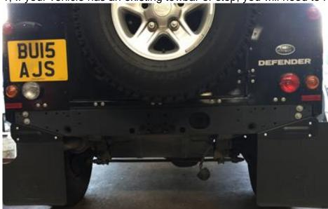
2, Clean the rear crossmember and prepare to fit your NAS. Remove the top left bolts from both sides of the crossmember.
