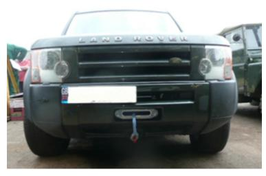
Prior to removing parts from your vehicle fit the winch into the mount.
