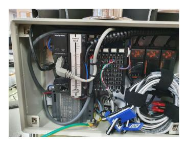
9) Each sensor cable is tagged with an ID label and is requires to be connected to its mating cable socket. Pay attention to the white dots indicating orientation of connection.
