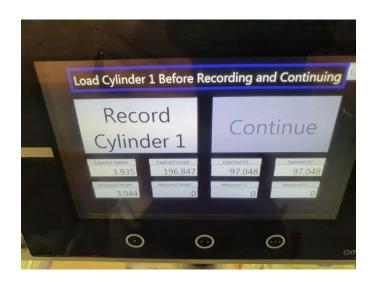
Place Master Cylinder 1 (97mm Diameter) on station ensuring sitting on all back tops and rotate slightly
