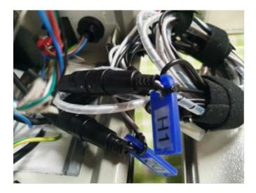
10) The Load cell cable needs to be passed through the same access port on the base of the control box and connected to the terminal block named with ID tagged wires to corresponding terminal position marked.
