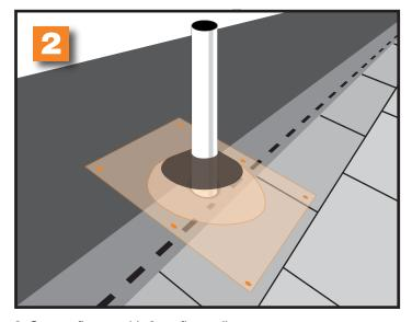
3. Secure flange with 6 roofing nails.
