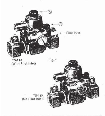
THE ROBERTSHAW "TS" SERIES THERMOMAGNETIC SAFETY VALVE is a control used to cut off the flow of gas to the burner in the event of pilot outage. The magnet assembly is energized by voltage generated by a thermocouple, that is heated by the pilot flame: When this flame is extinguished, the thermocouple voltage decreases until a spring overcomes the magnetic force and closes off both the pilot and main gas.
