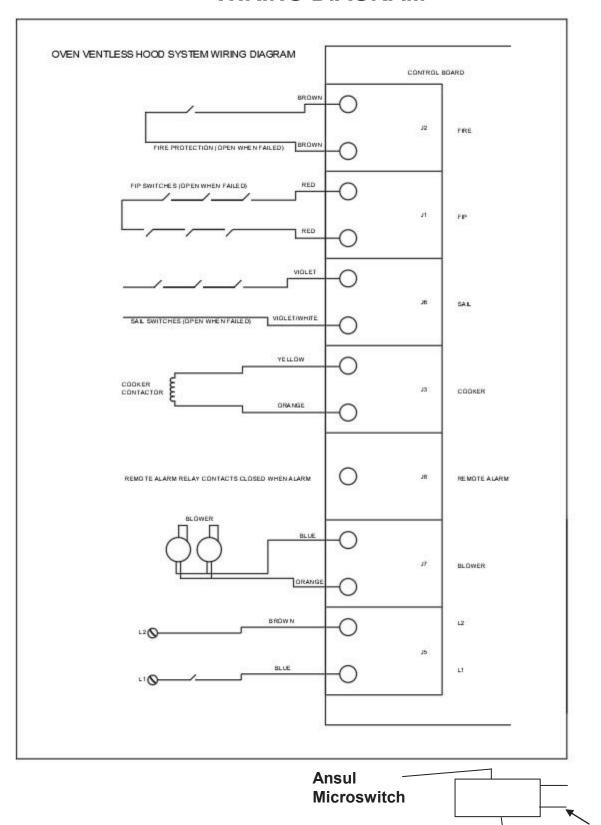
NOTE: PRIOR TO INSTALLATION, POWER MUST BE DISCONNECTED. WIRING DIAGRAM TO BE FOLLOWED IN ORDER TO INTEGRATE INTO FIRE SYSTEM. INSTALLATION SHALL BE PERFORMED TO MEET ALL STATE AND LOCAL CODES. ALL WIRING TO BE PER PAGES 7 & 8 OF THE INSTALLATION MANUAL.
