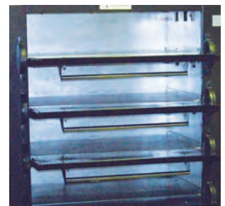
Adjustable Dampers at each deck
