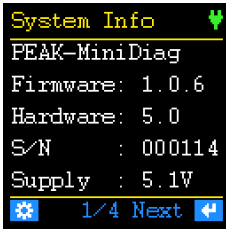
Indication of firmware and hardware version, serial number, and supply
