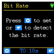
Automatic detection or manual configuration of the bit rate
