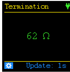
Measurement of correct termination
