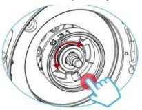
Note: For ease of adjustment and to protect the components, please hold down one side of the damping ring while using the other hand to turn the protruded part of the internal adjustment ring
