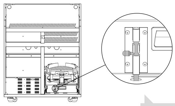
Be sure to secure the drawer by placing the locking cylinder in the hole in the floor.
