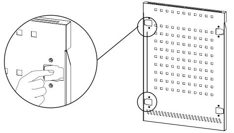
Be sure to break out the cover on the side of the door that corresponds to the opening direction.
