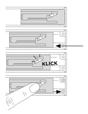
Snap the soft-close mechanism of the rail forward to tighten the rear two screws.
