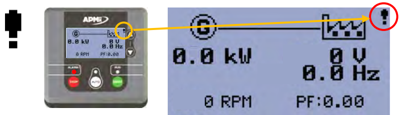
figure 14 - appearance of a fault
