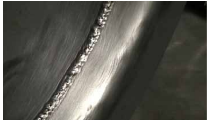
Step 3: Remove the tape to see a flat, well formed bead
