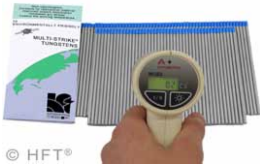
Radiation Monitor - low background radiation level
