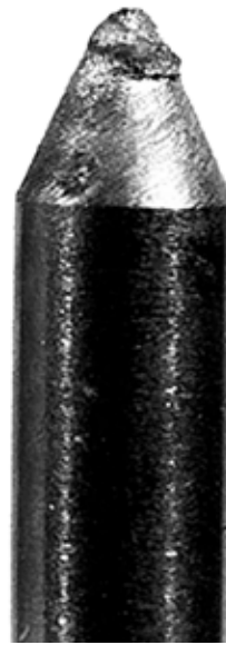
2% Thoriated Tungsten after 20 automatic welds
