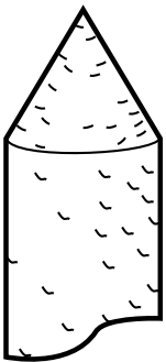
2% Thoriated Tungsten showing risk of uneven thorium distribution
