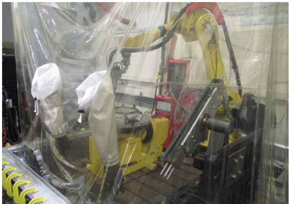
Flexible Welding Enclosure® for Titanium Additive Manufacturing
