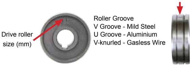
2 Open wire feed side panel and install wire into machine ensuring the drive roller is matched to the wire size and type. Refer to "Drive Feed Roller Selection" on page 16 Note: Wire to roll from under spool into wire feeder
