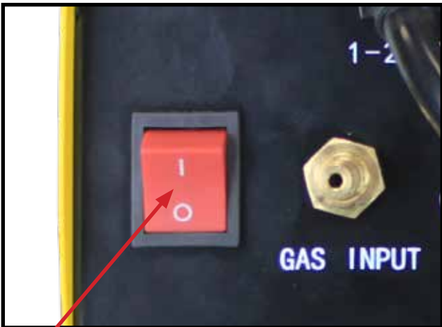
7 Switch the machine on using the mains power switch. Wait a few seconds whilst the machine powers up
