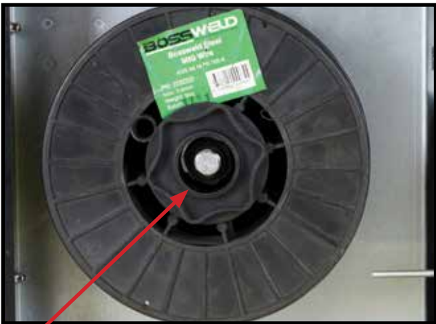
2 Open wire feed side panel and install wire into machine ensuring the drive roller is matched to the wire size and type. Refer to "Drive Feed Roller Selection" on page 16 Note: Wire to roll from under spool into wire feeder
