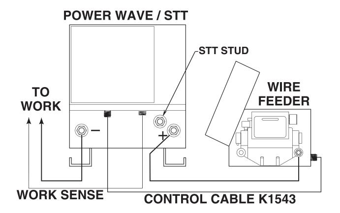
Connection Diagram Semi-automatic "Simple System" (Electrode Positive, STT® Configuration shown)
