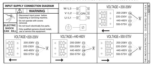
NOTE: Turn main input power to the machine OFF before performing connection procedure. Failure to do so will result in damage to the machine.
