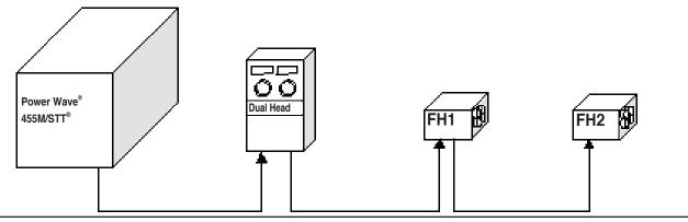
In this case the individual feed heads need to be assigned to the dual head control and the PW455 auto mapping disabled and the Equipment Groups set on (See figure A-6). (See the Feeder documentation for information on setting the feeder DIP switches)
