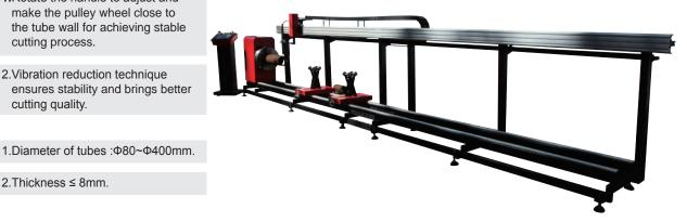
TubeTailor II is an economical CNC tube cutting machine with SteelTailor portable design. It is suitable for cutting tubes with diameter from 80 to 400mm and cutting various graphs in metal tubes, which have thickness of less than 8mm. Besides, it can work for different butt joint after welding tubes.
