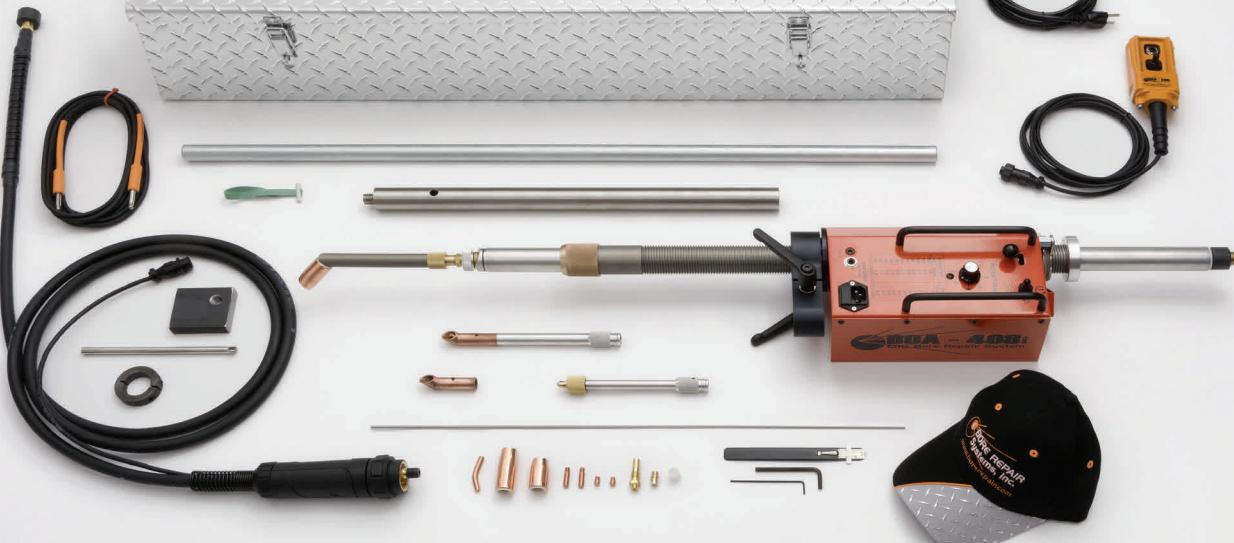
The BOA-408i automatic bore welding system is designed for users who demand durability, ease of setup and precision without unnecessary complication.
