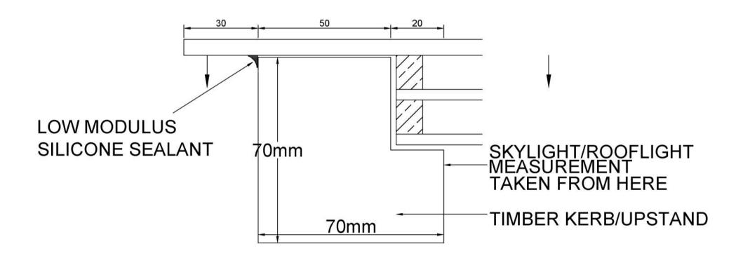
LOW MODULUS SEALANT MUST BE USED ANY SOLVENT BASED SILICONE SEALANT WILL INVALIDATE THE WARRANTY.
