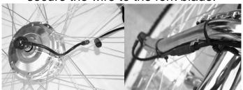
Route wires along the fork then along the bottom of the frame.
