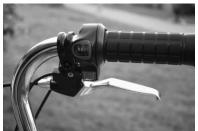
Attach brake cable to brake lever and connect to calipers. Tighten cable to ensure proper brake function.
