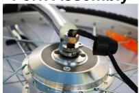
Loosen the headset and remove the original front fork from the frame. Mount new pre-assembled fork to the frame and tighten headset.
