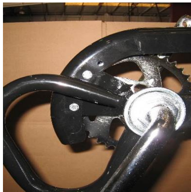
Front chainguard installation
