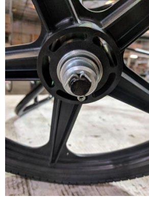
Outer washer, set collar and cotter pin
