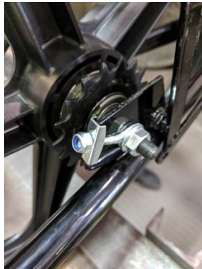
Wheel set into frame with accompanying hardware
