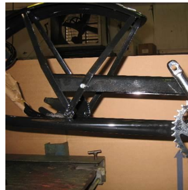
Rear chainguard installation
