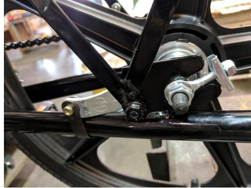
Front assembly completed, prior to chain adjuster being tightened
