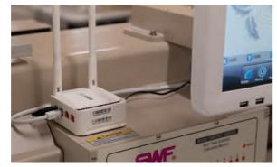
The KS Series machines offer Wi-fi capability for easy design transfer and remote monitoring of production progress and
