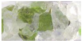
Grade 3 equivalent to 6mm gravel
