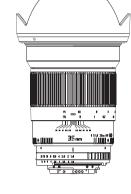
Align the attachment reference point on the hood with the reference point on the lens, push the hood onto the lens and turn the hood to the right until it makes a clicking sound.
