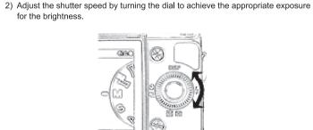
\* For some Sony E cameras, if you set the camera mode dial to A and set the brightness by turning the aperture adjustment ring on the lens, the camera automatically changes the shutter speed. Therefore you don't need to adjust the
