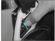
Replace the acoustic adapter plates by simply pressing them out with your thumb. Do it on both sides
