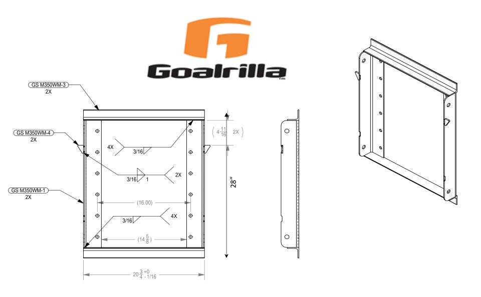
Wallmount Adjustable Bracket dimension 527mm(W) x 711mm(H)
