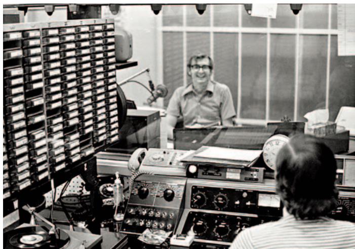
The biggest stations like KHJ (shown here) and WLS were unionized with a control board operator. In AM rock this allowed high production values with short songs, DJs, jingles and commercials flowing seamlessly, adding to the magic. A 45 RPM record is on the turntable at bottom left. The DJ in the distance is Johnny Williams who did all-nights for almost a decade (1965-74).
