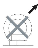
CAUTION: HOIST RING MUST BE FIRMLY SECURED TO OBJECT BEING LIFTED
