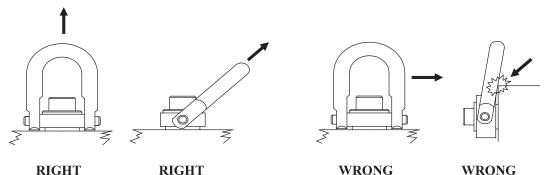
**Important**: The load on each hoist ring is not simply total weight divided by the number of hoist rings. The resultant force can be significantly greater at shallow lift angles and with unevenly distributed loads. See the example below.
