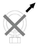
**Important:** The load on each hoist ring is not simply total weight divided by the number of hoist rings. The resultant force can be significantly greater at shallow lift angles and with unevenly distributed loads. See the example below.
