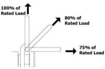
Important: The load on each hoist ring is not simply total weight divided by the number of hoist rings. The resultant force can be significantly greater at shallow lift angles and with unevenly distributed loads. See the example below.
