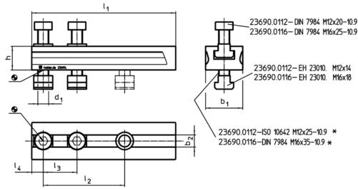
\* When using more height adaptors the screws ISO 10642 or DIN 7984 have to be replaced by screws extended by the dimension h.
