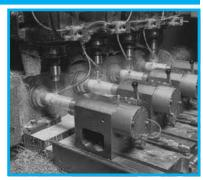
Special equipment spins ball bearings in place, then our ball cages move on to rigid quality inspection.
