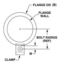
M = Flange OD to Clamp Bolt Center Bolt Radius = (Flange OD ÷ 2) + M
