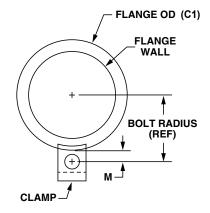
M = Flange OD to Clamp Bolt Center Bolt Radius = (Flange OD ÷ 2) + M
