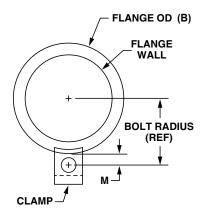
M = Flange OD to Clamp Bolt Center Bolt Radius = (Flange OD  $\div$  2) + M
