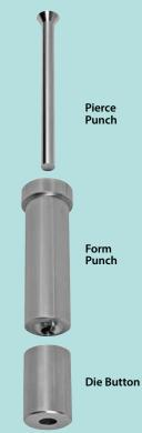
Dayton Thread Form Punch & Die Button Units (available in sets or as individual parts) offer you a single-step, in-die method for punching and forming threads. Dayton Thread Form Units offer many features and benefits over regular hole-tapping systems:
