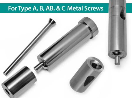
Dayton Thread Form Punch & Die Button Units offer you a single-step method for punching and forming threads. Dayton Thread Form works by punching the hole, lancing the material, and cutting a helical spiral in the material to form the proper thread helix for the desired type of metal screw. Thread Form creates a complete self-locking fastening system that holds the screws more tightly with metal tension—thereby reducing vibration, cutting assembly costs, and increasing productivity.
