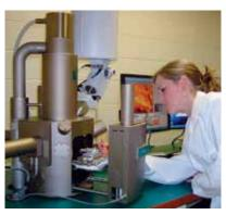
High-resolution scanning electron microscopes (above) and other devices are used to evaluate metal structures —often to determine the cause and prevention of product failure.
