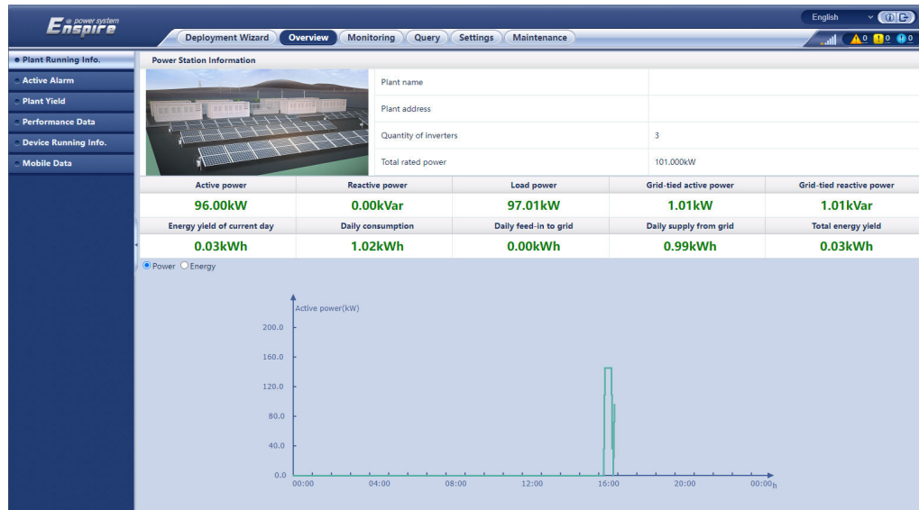
Figure 6-3 Plant running information (with power meter but without battery)
