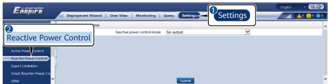
Figure 6-73 Reactive power control
