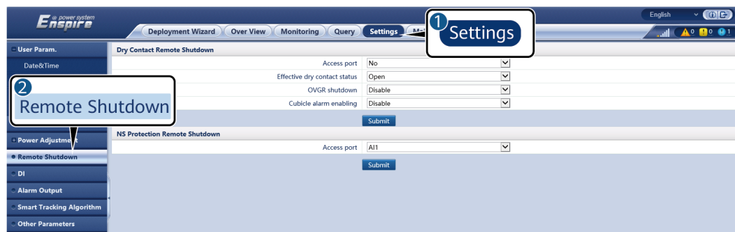
Figure 6-83 Dry contact remote shutdown
