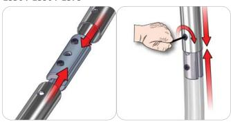
Compress the unlocked connector and slide one tube onto each end. Lock both screws carefully using your allen key tool. Be sure to lock securely, but do not overtighten.
