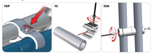
Be sure to fully assemble all frames before using clamps. With the clamp unlocked, place one tube of the first frame into the mouth of the clamp. Place the second tube (if applicable) into the second mouth of the clamp. With both frame's tubes in the clamp, be sure to lock securely, but do not overtighten.
