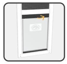
2. Loosen screws and open the metal strip/bar that clasps the flap in place
