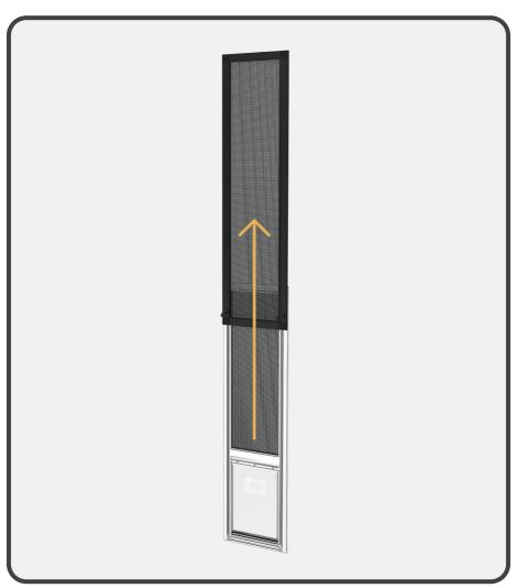
Insert pet door into sliding door track and slide up to extend, ensure a firm grip on door when extending/ retracting. Letting the top frame retract without guidance will cause damage to the door.
