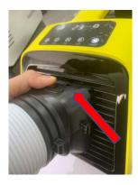
Front Connector and air duct Removal
