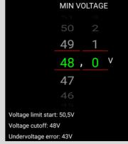
reached, the motor will stop and an UNDERVOLTAGE error will be displayed on the 1st screen of the App.
