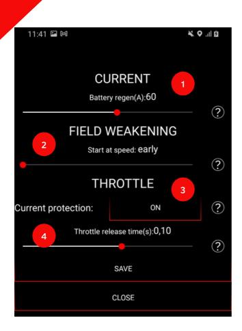
**<u>1-CURRENT-Battery regen:</u>** This option limits the max amount of current flowing back into the battery during regeneration. Adjust this setting based on your battery and the charging power capabilities of the battery.
