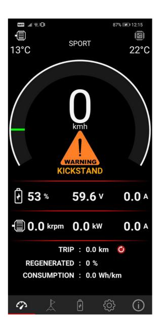
**IMPORTANT:** After the installation make sure to calibrate the throttle and Hall sensors! Go to the 5th screen of the Torp App and click the CALLIBRATION button. Then follow the setup Wizard. CALLIBRATION must be repeated after each firmware update!
