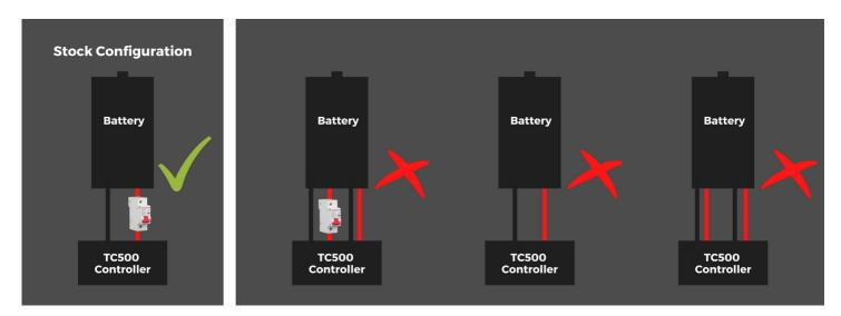
Use only tools and screws that came with the controller. Using the tools and screws that were not included in the parcel, not following these instructions, or not using the circuit breaker, can cause serious damage to you and your bike.
