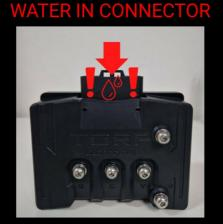
WARNING! Water in the main connector! Turn off the bike immediately, disconnect the main connector, and dry it out!
