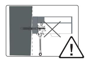
Please make sure the wall is straight and not wave. Warning: Don't tighten the nuts of the wall mount accessories too much otherwise it may cause breaking to the products.
