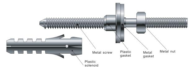
Note: These fixings are suitable for solid walls only. Plasterboard or stud walls may require specialist fixings (not supplied). Caution: care should be taken when drilling walls and floors to avoid anysunken wires or pipes
