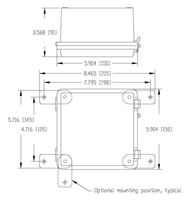
Figure 2: Small enclosure outline and mounting dimensions
