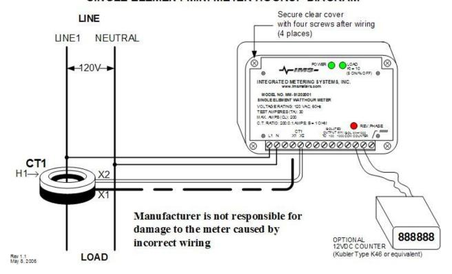
Figure 9: Mini Meter or EE Module hookup diagram
