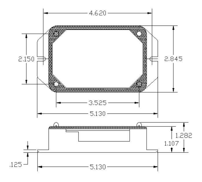
Figure 1: Single Mini Meter/EE Module case dimensions
