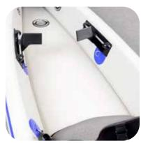
After inflation, adjust pedal for comfort and best bracing, raise pedal and slide it along the bar. Note setting number and match it on the other side.
