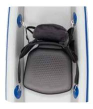
Using the seat straps, clip each strap to the D-rings. The upper straps attach to the forward D-rings.
