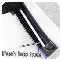
Bend the pad with one hand and pull rod into its hole with the other hand. If rod does not fully engage hole, release pad and use both hands to squeeze end of rod to pad until it slides in hole. Use care not to bend the rod.
