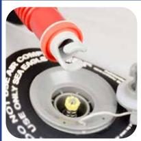
Check the hose end that goes in the board's valve. It should have hooks to lock it in the valve opening.
