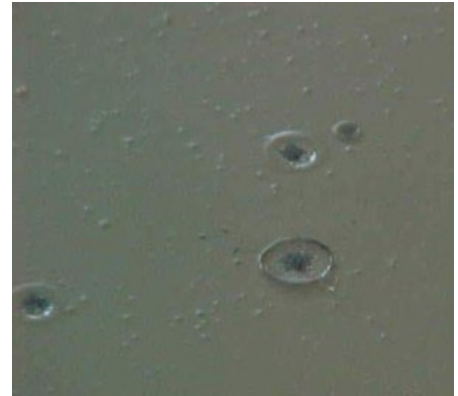
Pin Hole Craters left by popped bubbles
